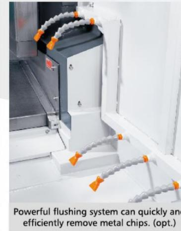
Powerful flushing system can quickly and efficiently remove metal chips. (opt.)
